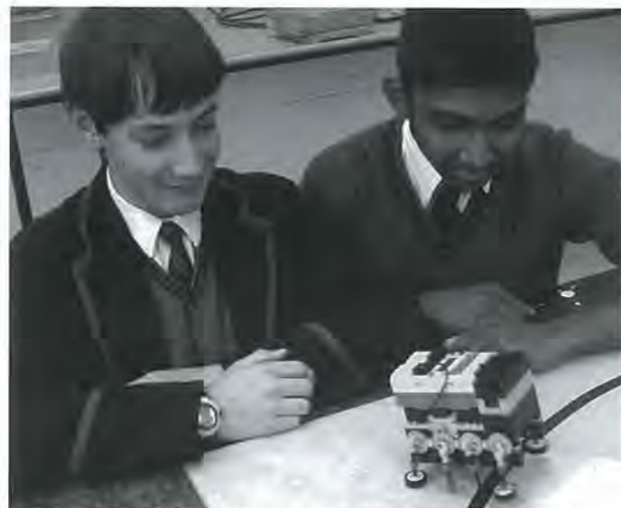
Peter Whitley and Eswaren Apparoo with their "Octopod" walking robot – mechanics to move over uneven terrain
