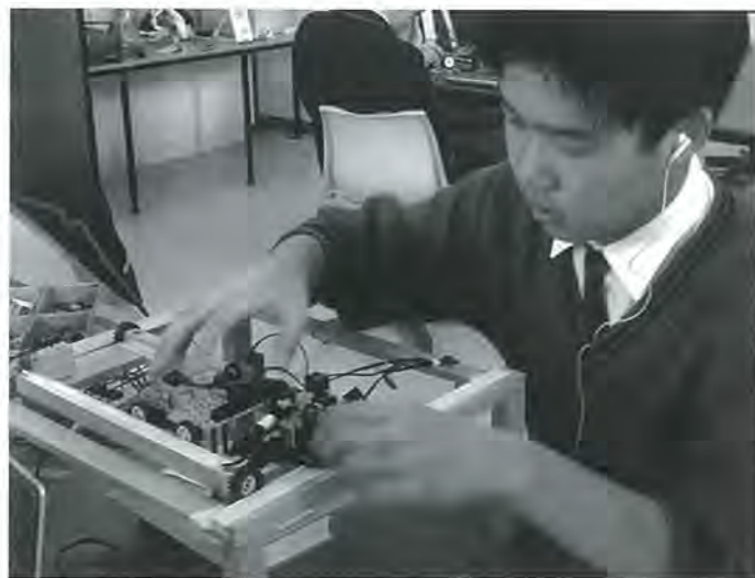
Matt Kang with his Tic Tac Toe playing robot – scans the game play and calculates its next move to prevent you from winning
