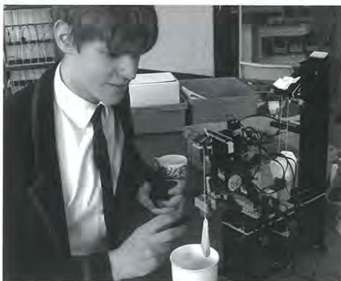
James Lord with his Tea making Robot – loads and dunks the teabag while monitoring the strength of the tea and tells you when the desired cup is ready
